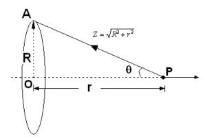
Figure shows a ring of mass M and radius R. Let P is the point at a distance r from the centre of the ring. By symmetry the field must be towards the centre that is along PO
