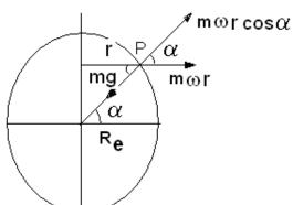
frame of reference. Everybody on its surface experiences a centrifugal force. Consider a point P . Perpendicular distance from point with axis of rotation is r . Then centrifugal force at point is  $m\omega^2 r \cos\alpha$ , going ouward where  $\alpha$  is the latitude of the place.
