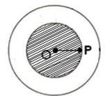
(ii) Gravitational field at point inside the sphere is only due to the mass enclosed by the surface passing through the point, volume enclosed is shown by shaded portion in diagram and field due to outer volume is zero.
