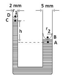
each surface exceeds that on the convex side by 2T/r, where T is surface tension and r is the radius of the limb concerned Now  $r_1$  = 2.5 mm = 2.5×10<sup>-3</sup> m and  $r_2$  = 1mm = 10<sup>-3</sup>m Hence
