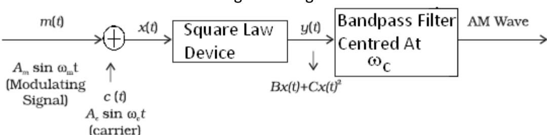
Here the modulating signal  $A_m \sin \omega_m t$  is added to the carrier signal  $A_c \sin \omega_c t$  to produce the signal  $x(t) = A_m \sin \omega_m t + A_c \sin \omega_c t$  is passed through a square law device which is a non-linear device which produces an output
