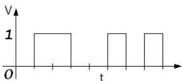
One can show that this rectangular wave can be composed into a superposition of sinusoidal waves of frequencies  $v_0, 2v_0, 3v_0, 4v_0 \dots nv_0$  where n is an integer extending to infinity and  $v_0 = 1/T_0$ . The fundamental ( $v_0$ ), fundamental ( $v_0$ ) + second harmonic ( $2v_0$ ), and fundamental ( $v_0$ ) + second harmonic ( $2v_0$ ) + third harmonic ( $3v_0$ ), are shown in the same figure to illustrate this fact.
