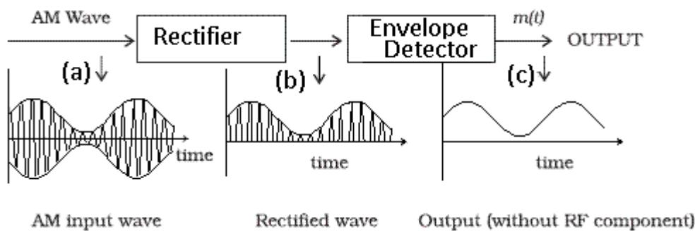
The modulated signal of the form given in (a) of fig. is passed through a rectifier to produce the output shown in (b).
