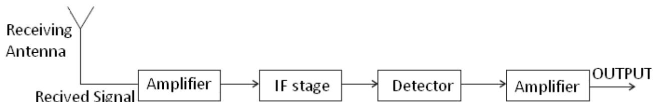
The detected signal may not be strong enough to be made use of and hence is required to be amplified. A block diagram of a typical receiver is shown in Detection is the process of recovering the modulating signal from the modulated carrier wave.
